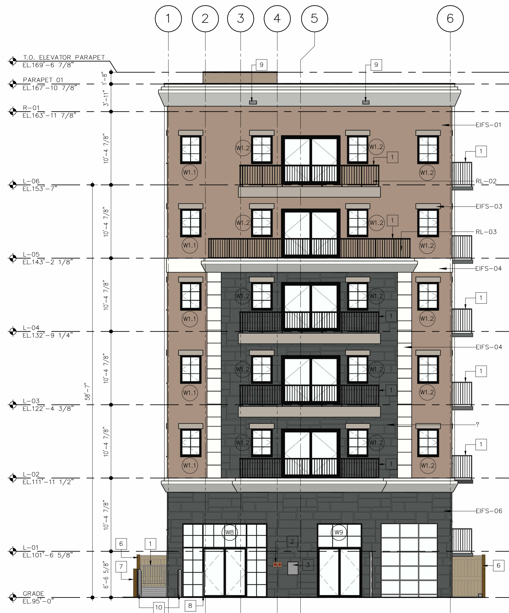
1 A4.1 EXTERIOR BUILDING ELEVATION - SOUTH 1/8" = 1'-0"
