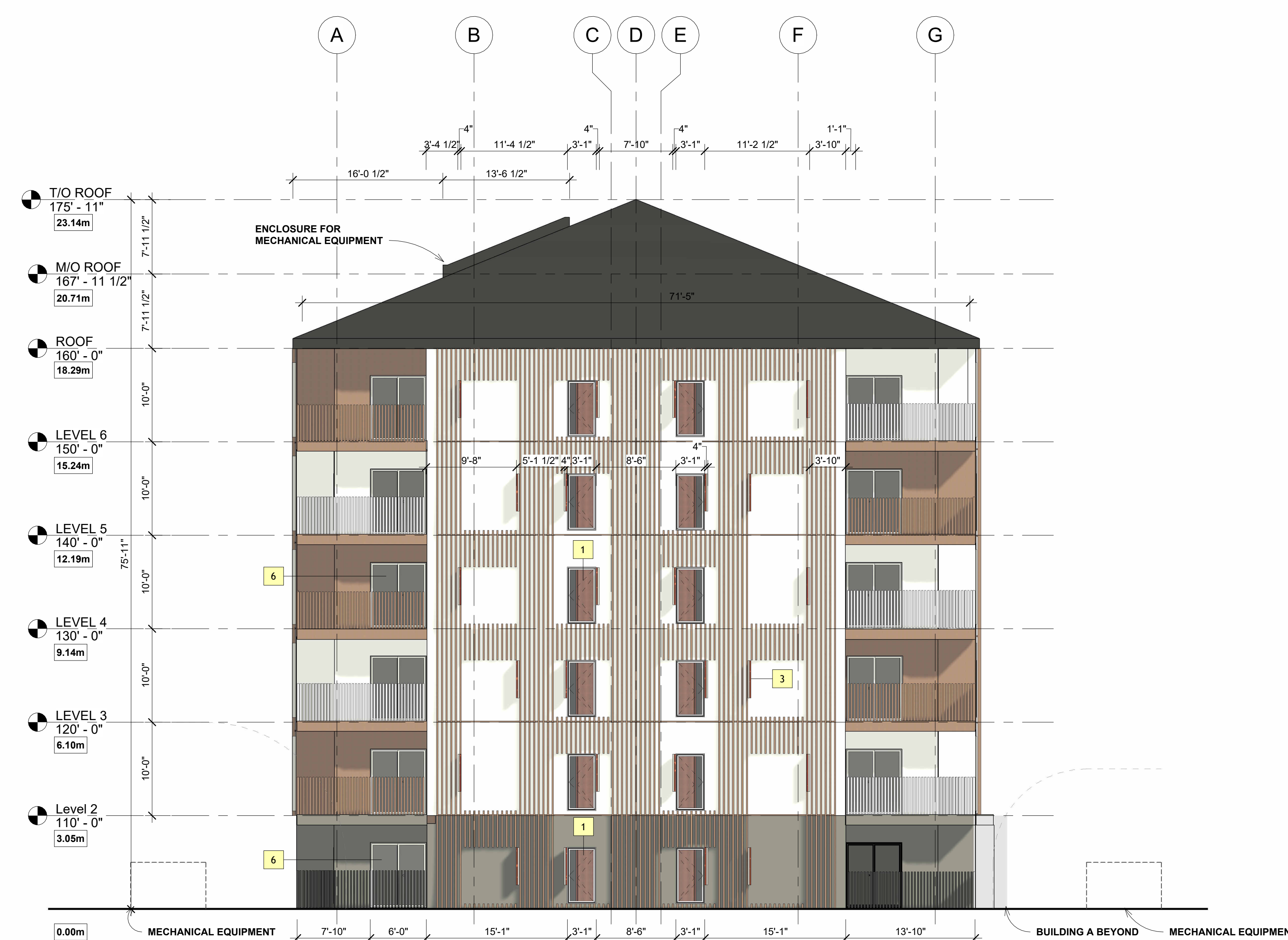
1 WEST BUILDING WEST ELEVATION A-260-3.0 1/8" = 1'-0"
