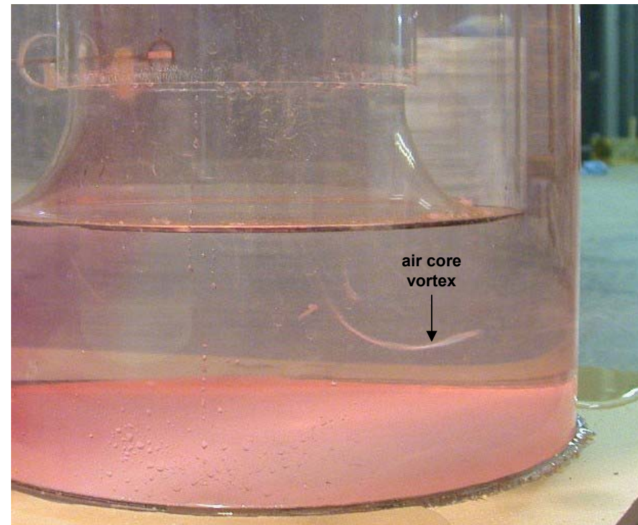
2) View of a Type 5 subsurface air core vortices that formed on the sidewall of the pump can at locations approximately 60 degrees on either side of the inlet. Type 3 subsurface vortices also formed on the can wall directly opposite the inlet at approximately bell level. (16506-007)
