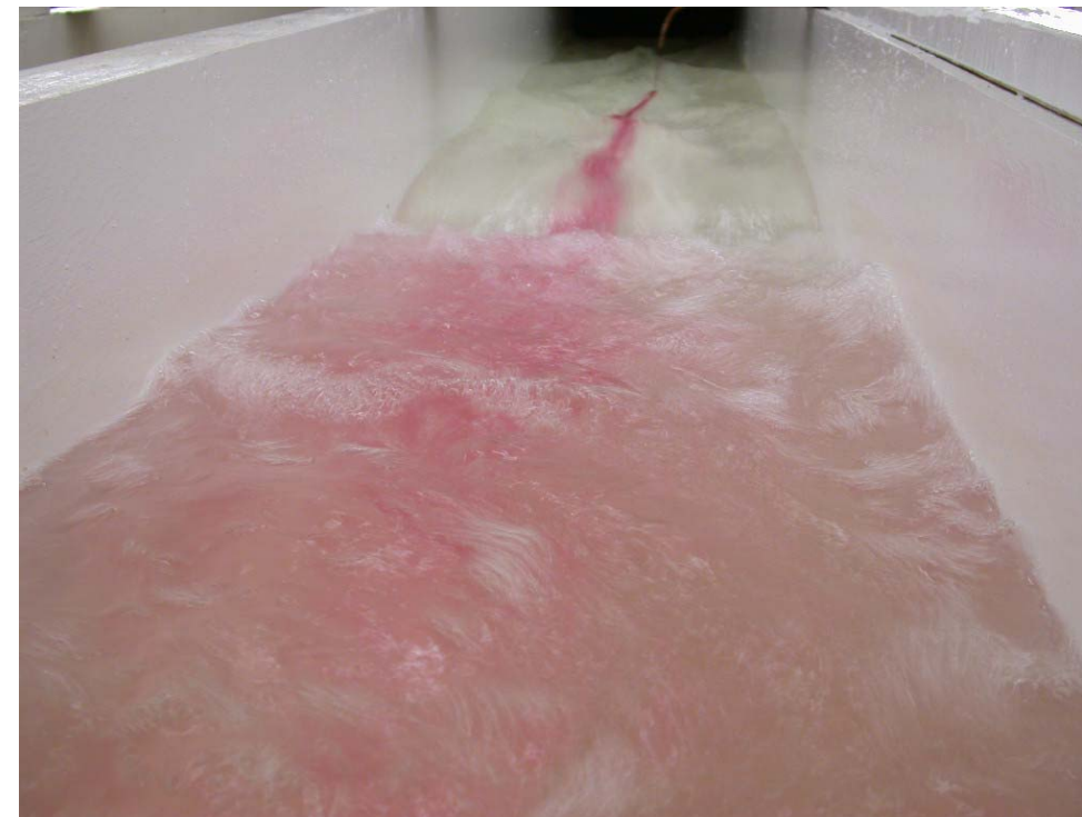
4) View looking upstream at the effluent conduit. For three and four-pump operation at low water level, a hydraulic jump formed on the sloping transition. The hydraulic jump created a significant amount of turbulence and entrained air bubbles that entered the pumps. (16506-004)
