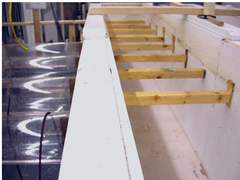
1) View looking downstream in the conduit at the recommended seven square vortex breaker bars that were installed with their tops at El. 4.25 m. (16506-008)
