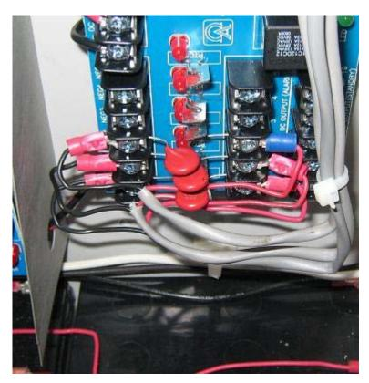
.7 Wires and modules inside the controller's enclosures shall be labeled. Wires shall be secured inside the enclosure using Ty-raps and adhesive backed mounting brackets. Enough cable slack should be left for servicing the hardware modules.
