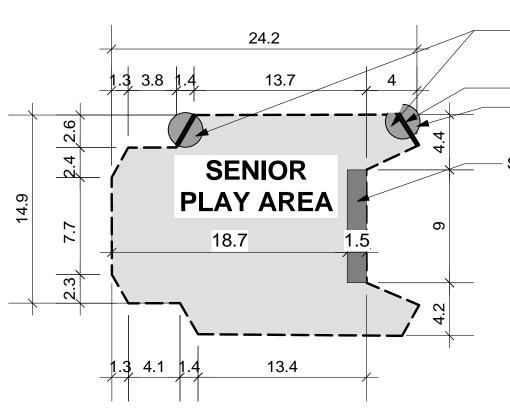
No Play Equipment protective surfacing zone within this area (sloped Wood Fibre to meet safety surfacing grade).
