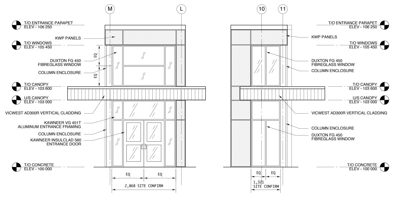
NOTE: TEMPERED GLASS WITH 6mm AND SULL SASH FOR ALL VESTIBULE GLAZING
