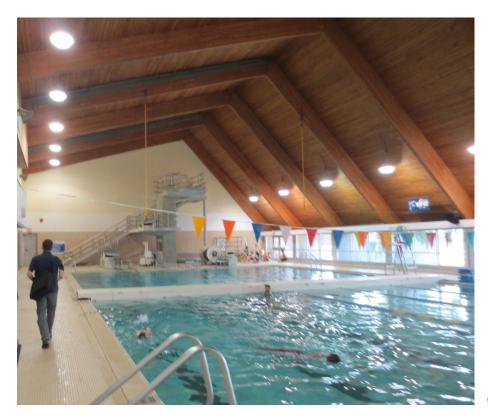
Left: The interior of the Pool Area. The dramatic roof structure is comprised of glued, laminated beams and solid fir decking
