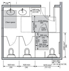
NOTE: In a retrofit situation where it is technically not feasible to provide the required clearances, the dimension marked with an \* may be reduced to 1525 mm (60 in.).
