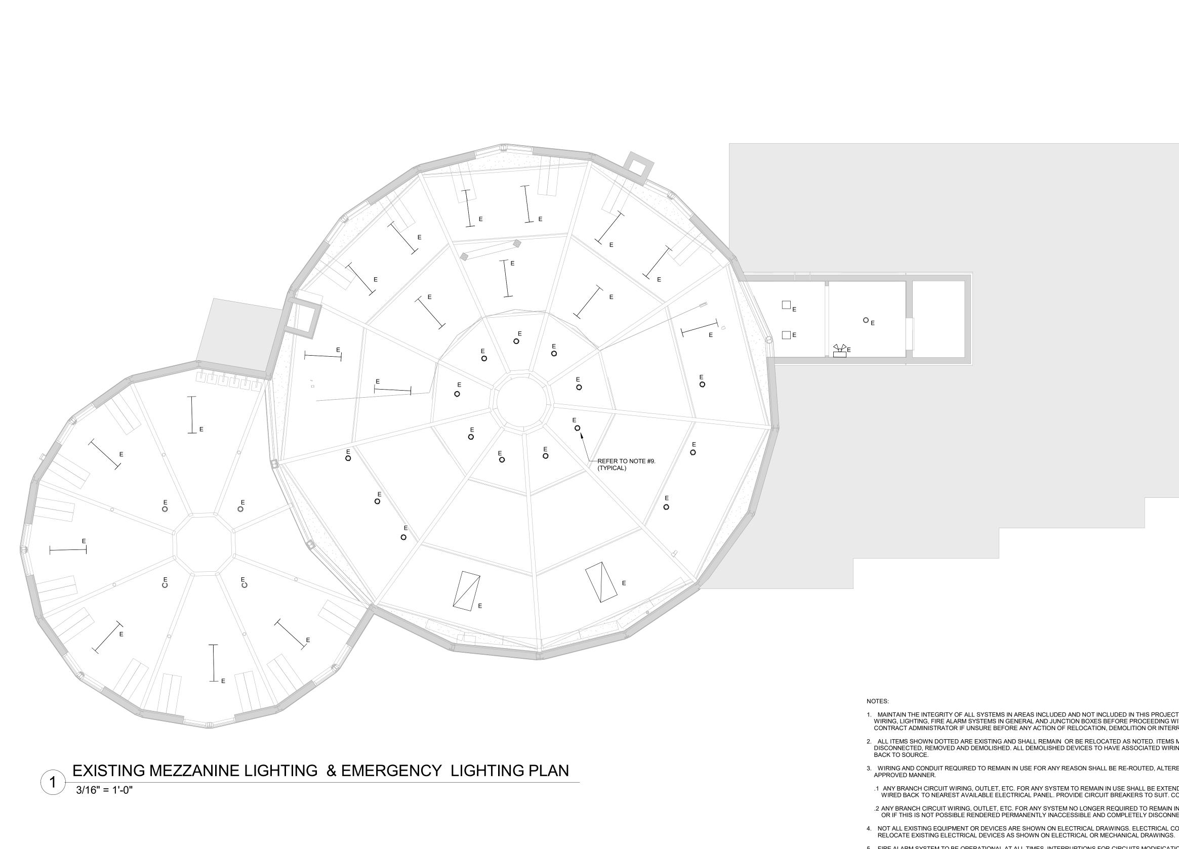
8. ALL EXISTING LIGHT SWITCHES IN DRYWALL WALLS TO BE LOWERED TO 1000mm AFF. EXTEND, RE-ROUTE, RE-WIRE AND RECONNECT AS  $\sim$
