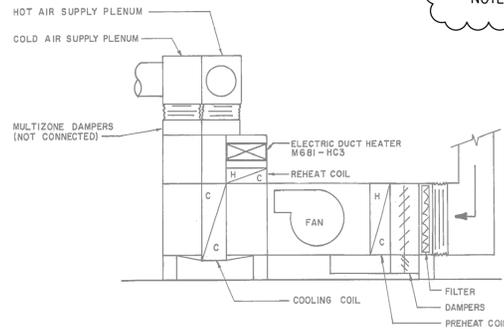
AIR HANDLING UNIT M681-F81 ELEVATION
