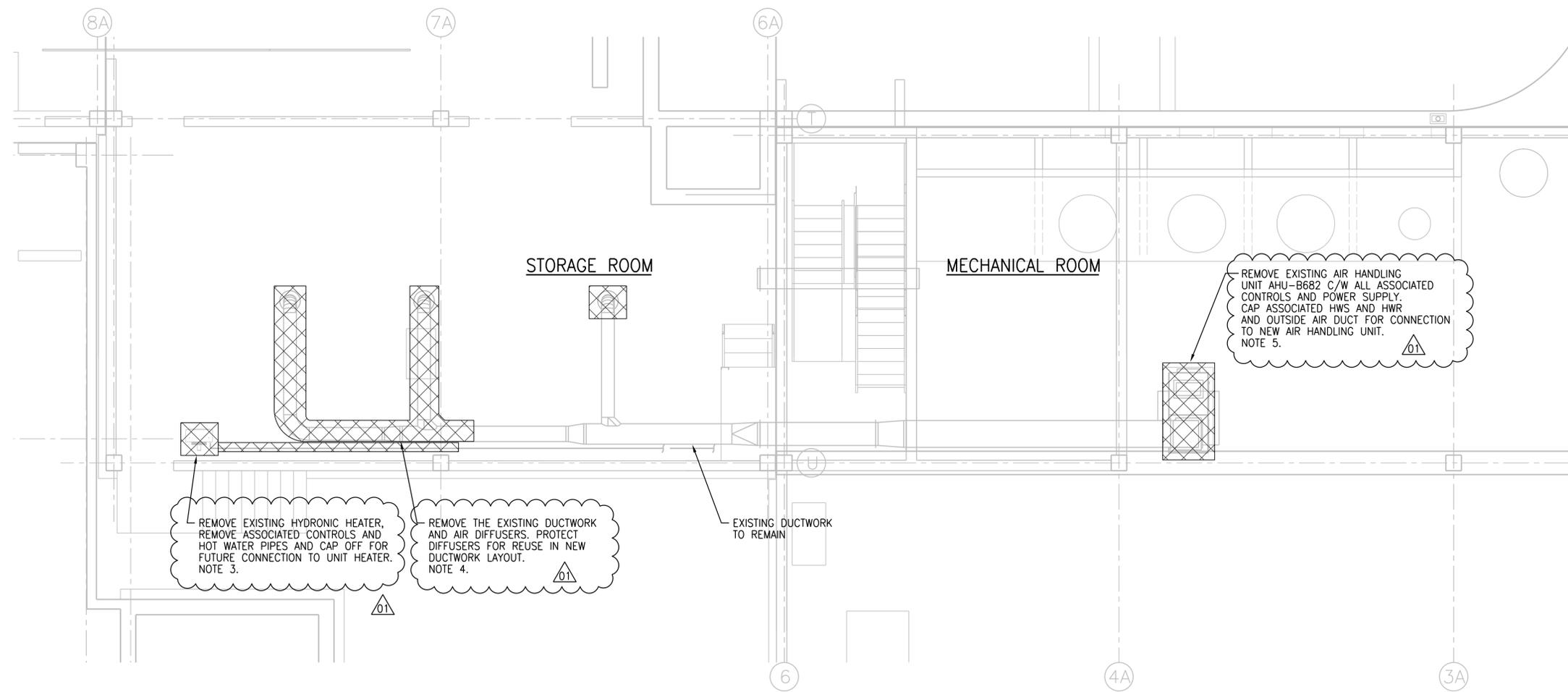
REMOVE EXISTING HYDRONIC HEATER, REMOVE ASSOCIATED CONTROLS AND HOT WATER PIPES AND CAP OFF FOR FUTURE CONNECTION TO UNIT HEATER. NOTE 3.
