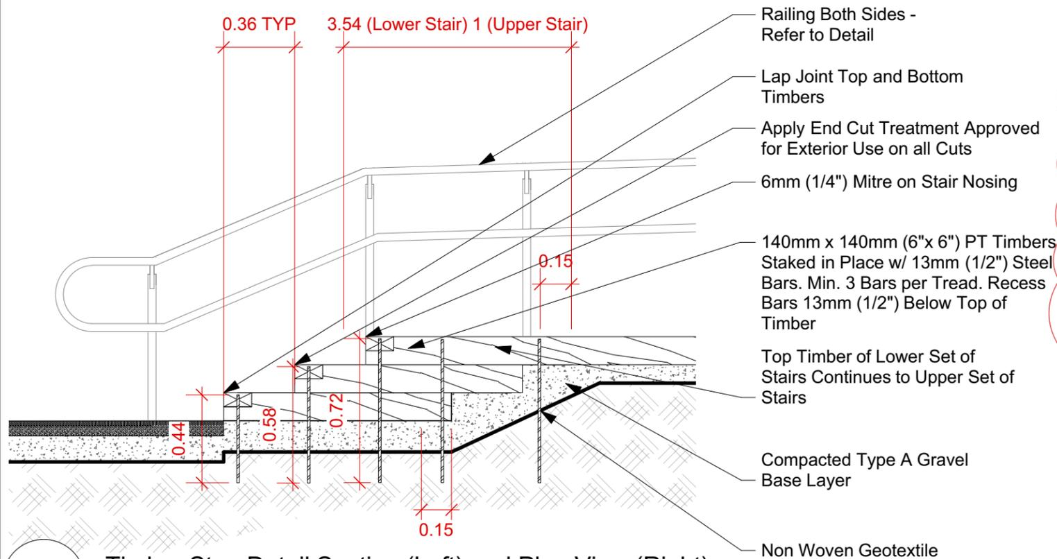
2 Timber Step Detail Section (Left) and Plan View (Right)
