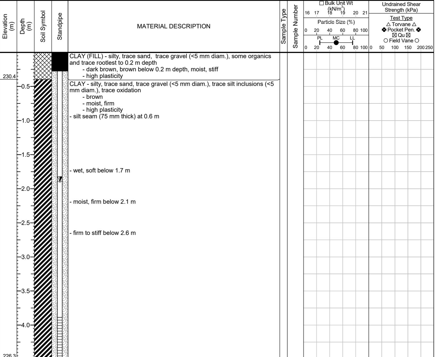
END OF TEST HOLE AT 4.5 m IN CLAY
