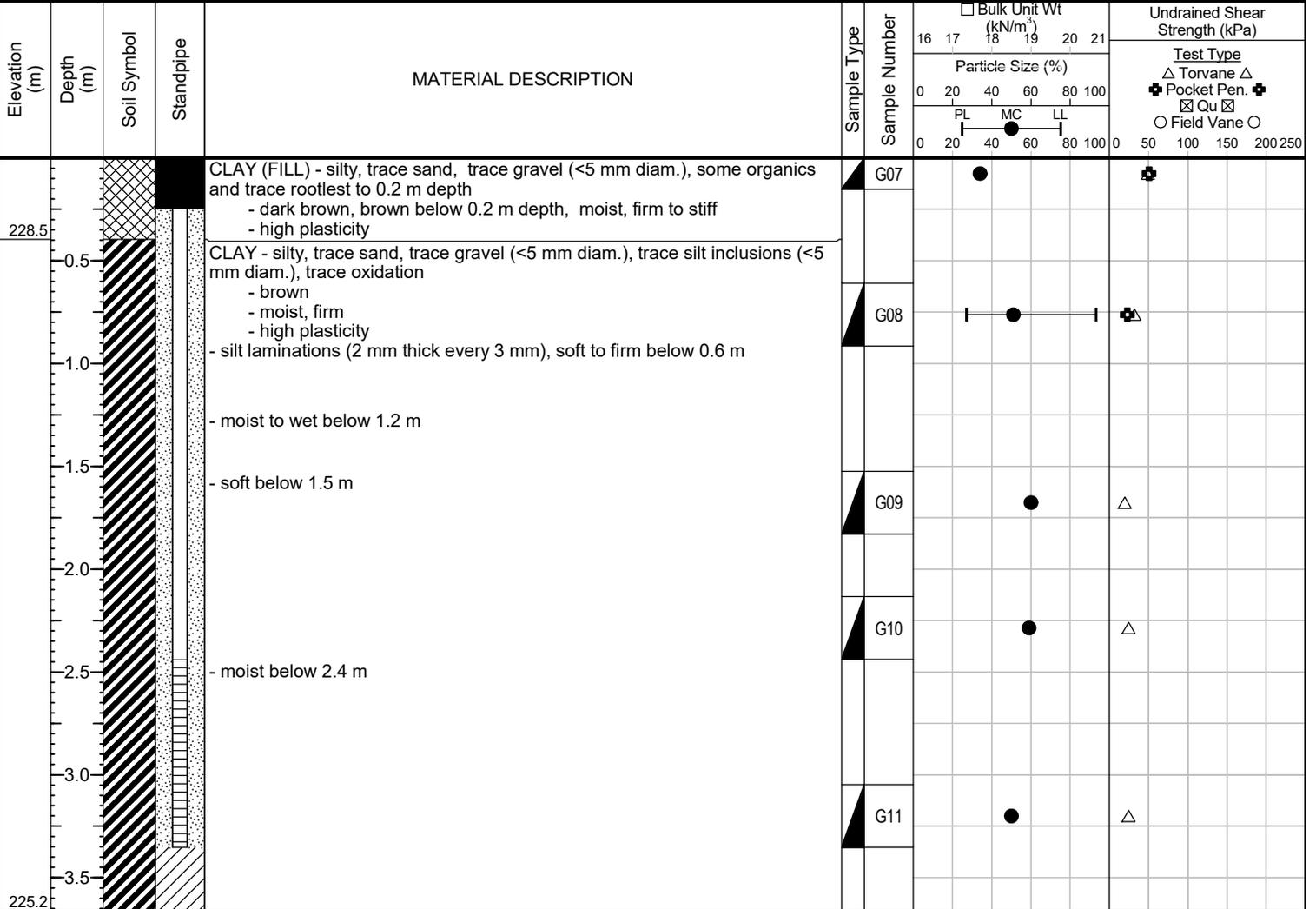
END OF TEST HOLE AT 3.7 m IN CLAY
