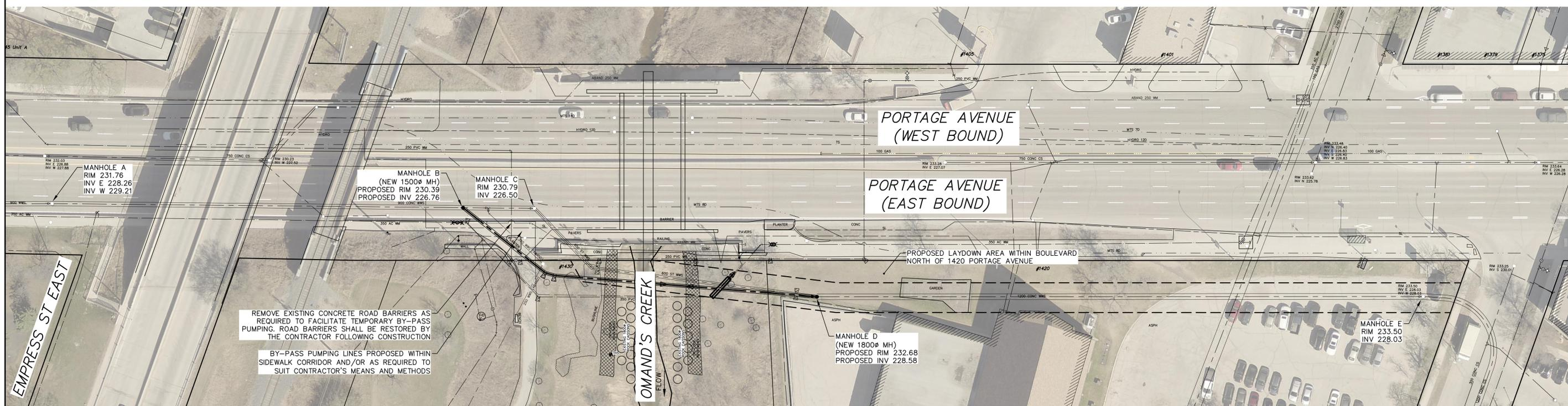
REMOVE EXISTING CONCRETE ROAD BARRIERS AS REQUIRED TO FACILITATE TEMPORARY BY-PASS PUMPING. ROAD BARRIERS SHALL BE RESTORED BY THE CONTRACTOR FOLLOWING CONSTRUCTION
