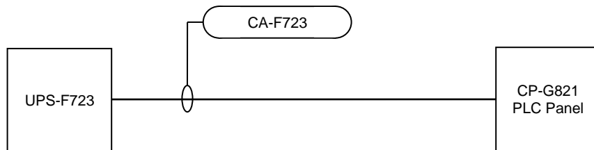
Figure 7-3: Instrument Cable Identification Example – Identified Equipment
