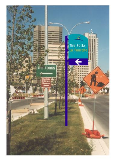
In median in front of light pole. Sign edge 2' from curb edge. Remove existing signs in median.
