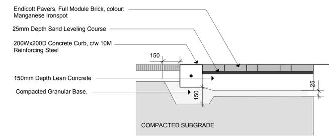
3 Unit Pavers on Lean Concrete Base - Section
