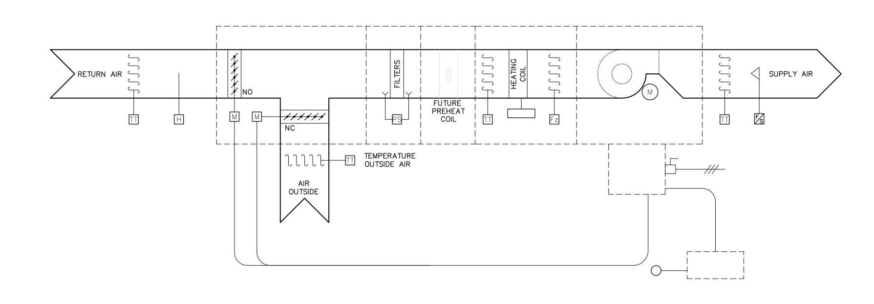
SCHEMATIC - INLET BUILDING AHU-2
