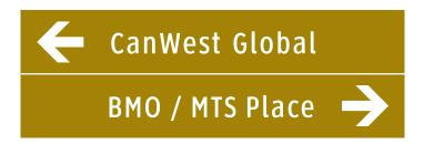
Notes: Insert to fit on existing lit sign 12"x36". See photo CN1 for typical installation.
