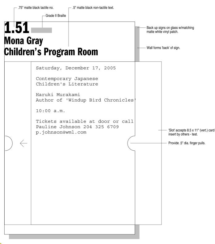
Type H.9T: .25± x 8.5" x 14.35" non-glare acrylic w/tactile no. + Braille, + non-tactile text; slot, VHB adhesive. Centre on wall or sidelite 2" from door frame on latch side, 48" AFF. Sim. for: '2.27 Buchwald Room'; '2.28 Anhang Room'; '2.35 Carol Shields Memorial Auditorium'; '2.45 Meeting Room 2'; '2.59 Tutorial A'; 2.59A Tutorial B'; '2.60 Meeting Room 1'.
