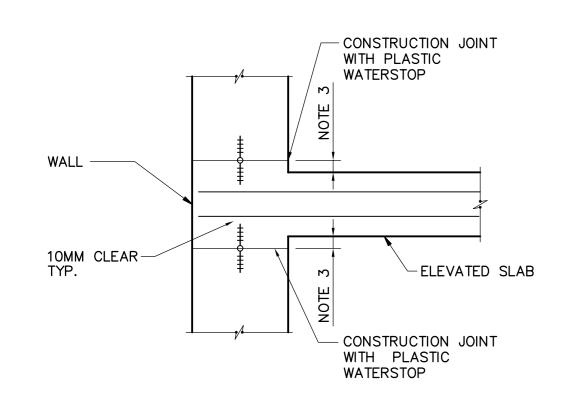
1. FOR SLAB CONCRETE COVER, SEE 2. FOR SIZE OF WATERSTOP SEE / 1 WB-S0446
