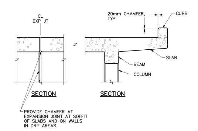
PROVIDE CHAMFER ALONG EXPOSED EDGES ON CONCRETE SLABS, BEAMS, CURBS, COLUMNS, WALL OPENINGS AND SIMILAR ITEMS UNLESS OTHERWISE NOTED OR DIRECTED.
