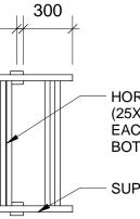
HORIZONTAL PICKET RAIL (25X25mm) (LINE UP WITH EACH CIRCLE) WELD TO BOTTOM RAIL
