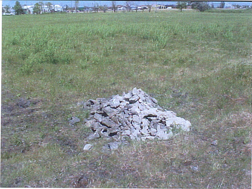
PHOTO #3- GEOTECHNICAL TEST HOLE CUTTINGS
