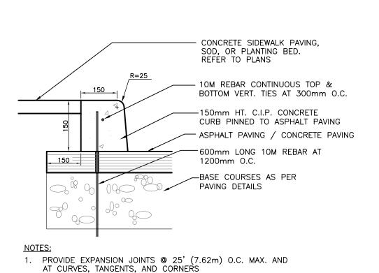
BASE OF CURB TO REST ON ASPHALT PAVING
