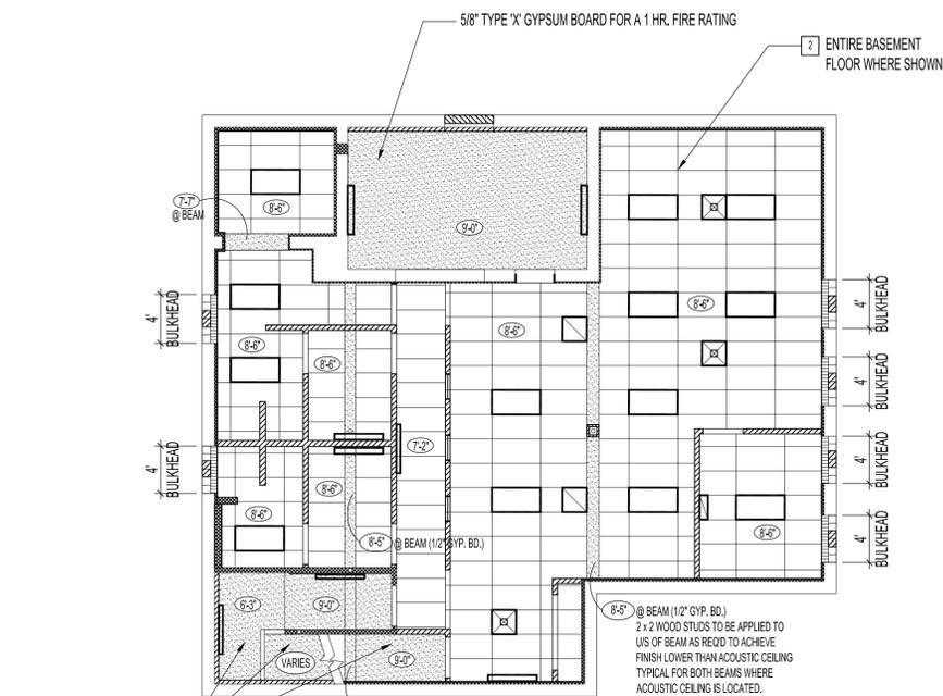
**BASEMENT FLOOR PLAN - REFLECTED CEILING PLAN**
