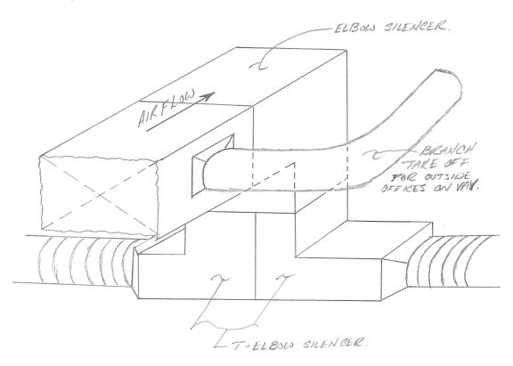
**2.** The duct work transitions from AHU-1 near gridline A.2 shown in the photograph below are to be reworked using acoustic plenums. Refer to the attached sketch below.
