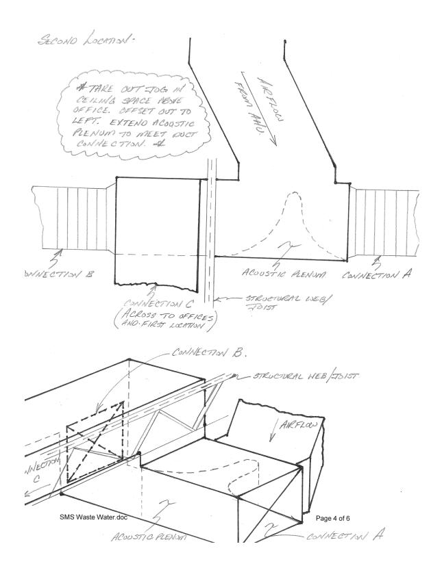
**3.** The discharge plenum for AHU-2 located between gridlines B and C is to be revised. Provide minimum 18 gauge acoustically lined ductwork for the new plenum, revise provide elbow silencers at each of the two elbows from the plenum. Ductwork connected to the plenum via flexible connections.
