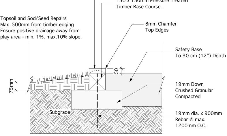
Base course timbers shall be pinned with minimum of two (2) 19mm dia, rebar @ max. 1200mm O.C. Top course shall be screwed down using screws treated for ACQ use and sized to suit. Two screws at each end and every 600mm alternating sides along length. Screws shall be Robertson #8 63.5mm (2 \_") yellow zinc plated. Min. length of timbers to be 1200mm. Install longest lengths possible.
