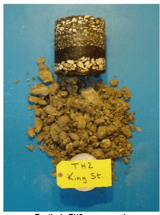
Testhole TH2 core sample
