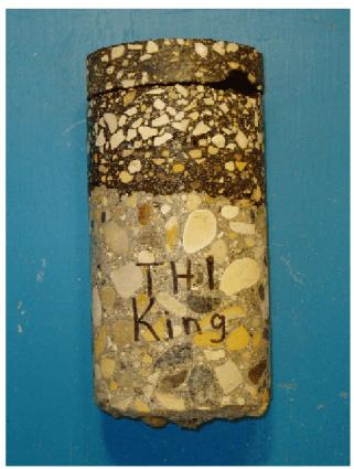
Testhole TH1A core sample
