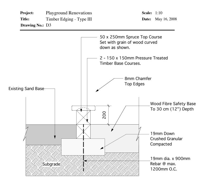
Base course timbers shall be pinned with minimum of two (2) 19mm dia, rebar @ max. 1200mm O.C. Timber above base course shall be securely spiked with min. two 12mm dia. x 250mm spikes @ max. 1200mm O.C. Top course shall be screwed down using screws treated for ACQ use and sized to suit. Two screws at each end and every 600mm alternating sides along length. Min. length of timbers to be 1200mm. Install longest lengths possible.
