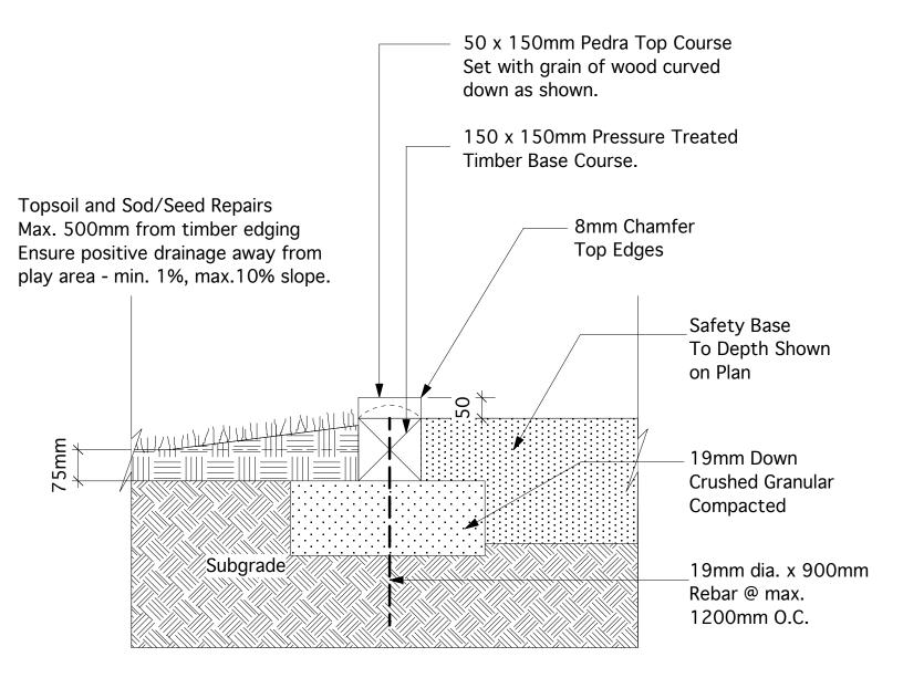
Base course timbers shall be pinned with minimum of two (2) 19mm dia, rebar @ max. 1200mm O.C.
