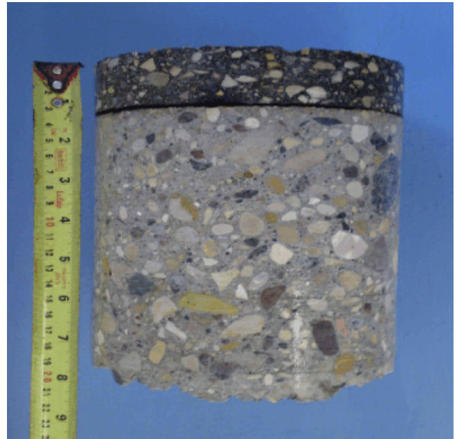
Pavement core from Testhole TH 2
