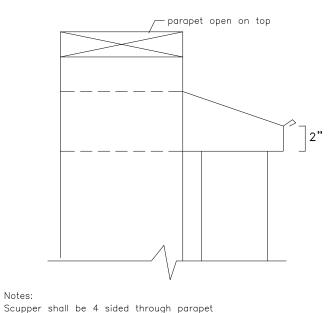
Note: Details are to be similar for inverted roof assemblies
