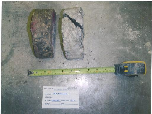
Photo 9: Asphalt core sample from TH-09-08
