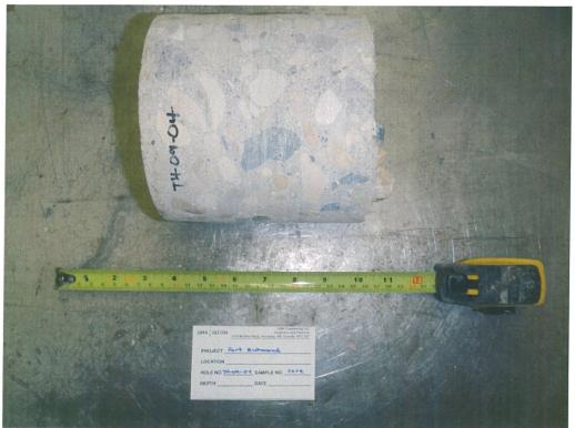
Photo 4: Concrete core sample from TH-09-04
