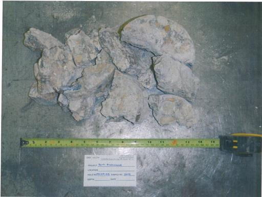
Photo 5: Concrete core sample from TH-09-05
