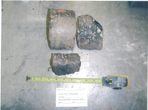
Photo 7: Asphalt core sample from TH-09-07
