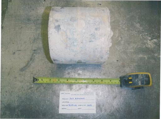
Photo 6: Concrete core sample from TH-09-06
