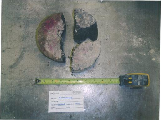
Photo 10: Asphalt core sample from TH-09-08
