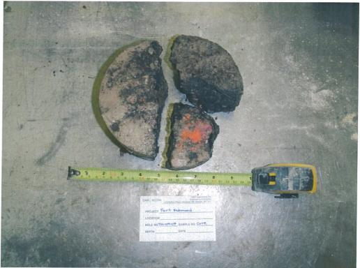
Photo 8: Asphalt core sample from TH-09-07
