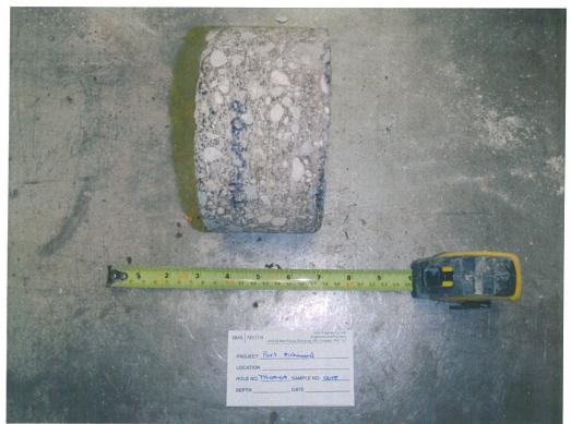
Photo 11: Asphalt core sample from TH-09-09
