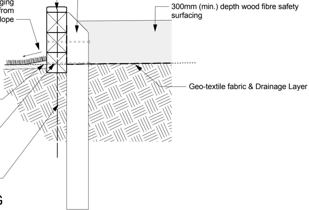
300mm (min.) depth wood fibre safety surfacing
