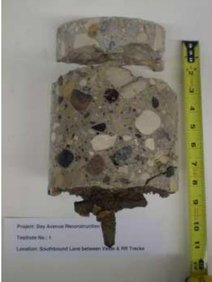
**Photo 1:** Testhole D1: Southbound Lane between Valle & RR Tracks
