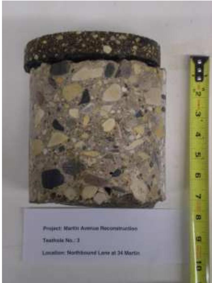
**Photo 18:** Testhole M3: Northbound Lane at 34 Martin
