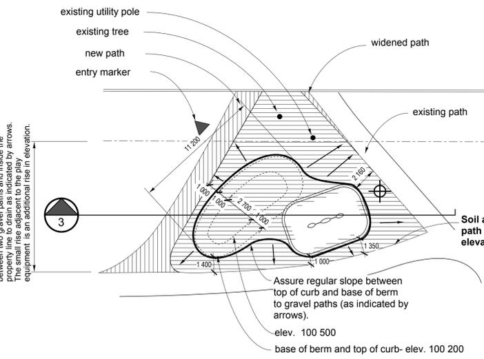
**2 plan 1: 200** note: 7 stumps must be removed in this area
