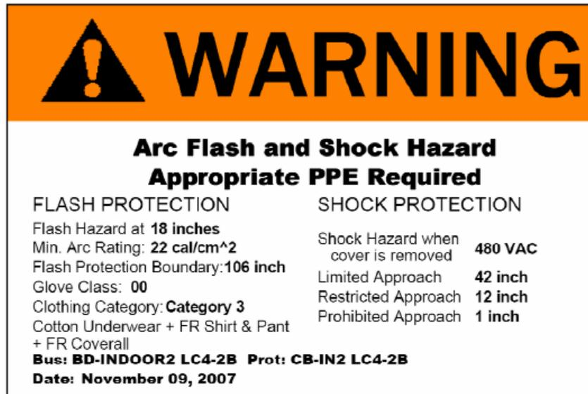
Figure 1 – Example of Arc Flash Warning Label
