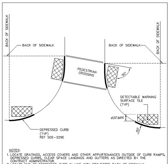
2. LOCATE END OF DEPRESSED CURB IN LINE WITH PROJECTED BACK OF SIDEWALK.
