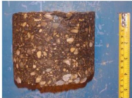
Core sample from Testhole TH2
