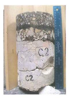
Charles Street TH #2 0 mm to 35 mm Asphalt (newer) 35 mm to 80 mm Asphalt (older) 80 mm to 240 mm Concrete
