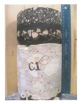
Charles Street TH #1 0 mm to 40 mm Asphalt (newer) 40 mm to 85 mm Asphalt (older) 85 mm to 230 mm Concrete
