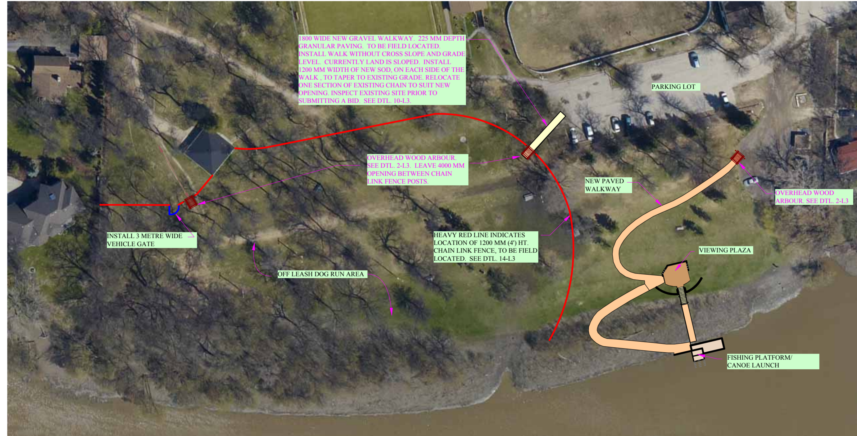
1 SCHEMATIC LOCATION OF NEW CHAIN LINK FENCE AND ARBOUR LOCATIONS Scale: N.T.S.
