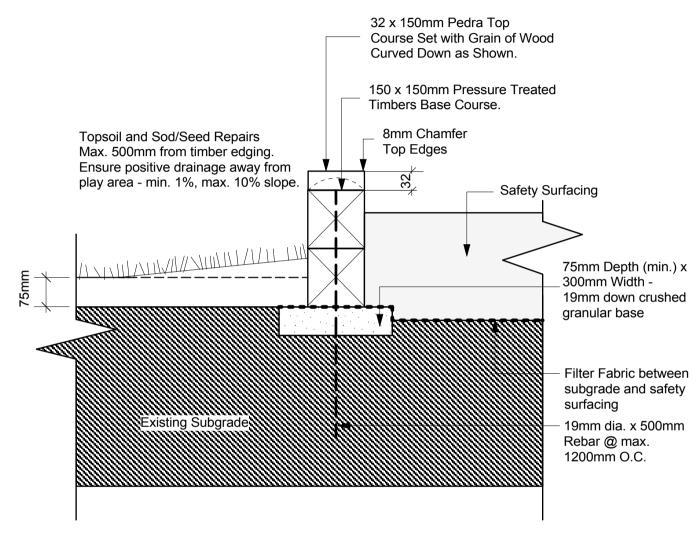
Base course timber shall be pinned with minimum of two (2) 19mm dia. rebar @ max. 1200mm O.C. Pedra top course shall be pre-drilled and screwed down using screws treated for ACQ use and sized to suit. Two screws at each end and every 600mm alternating sides along length. Only use but joints for straight sections of pedra. Min. length of timbers to be 1200mm. Install longest lengths possible.
