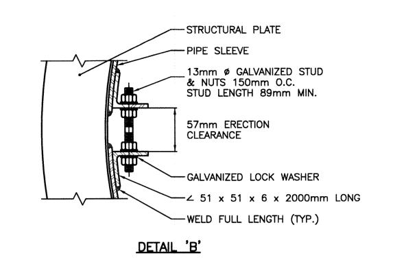
INTERNAL SLIP JOINT DETAILS SCALE: N.T.S.
