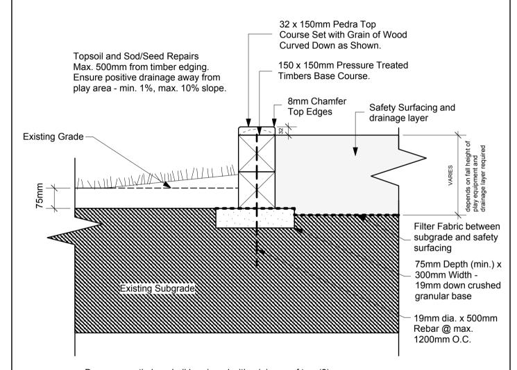
Base course timber shall be pinned with minimum of two (2) 19mm dia. rebar @ max. 1200mm O.C.
