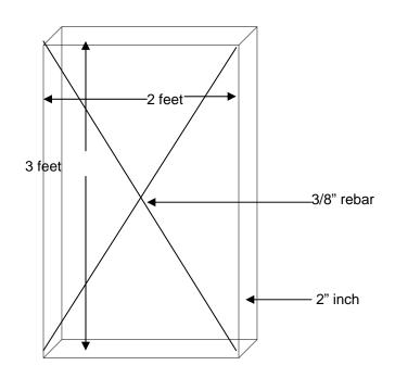
Note: 3/8" (inches) rebar to be used as illustrated; to reinforce the concrete non-slip surface is required.
