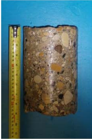
Core sample from Testhole TH1
