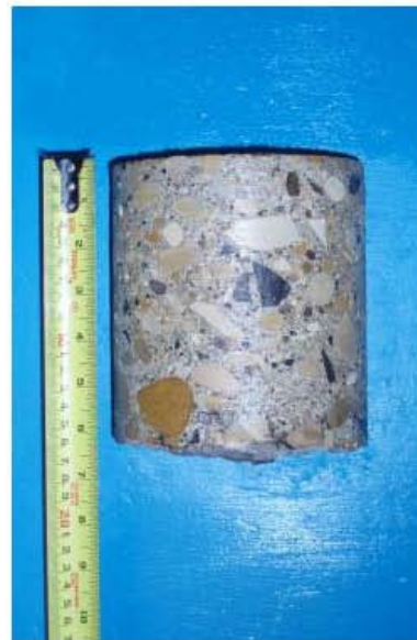
Core sample from Testhole TH4
