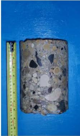
Core sample from Testhole TH5
