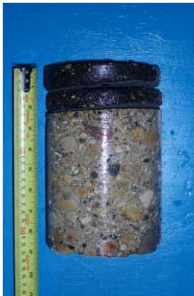
Core sample from Testhole TH3
