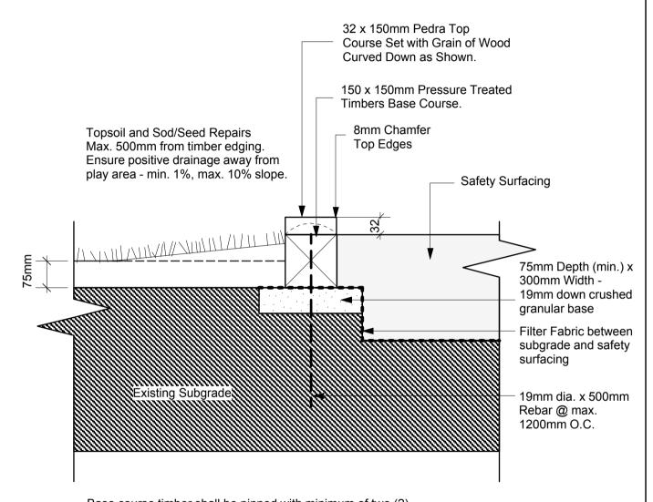
Base course timber shall be pinned with minimum of two (2) 19mm dia. rebar @ max. 1200mm O.C. Pedra top course shall be pre-drilled and screwed down using screws treated for ACQ use and sized to suit. Two screws at each end and every 600mm opposite sides along length. Only use but
