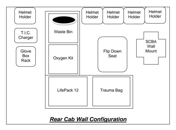
NOTE: Interior Storage Compartment on rear wall of cab beside flip up seat to contain equipment: Cabinet to be made of metal -dimensions approximately 36" wide under seat, and 15" wide, full height of cab with 4 latching doors (see attached drawing) All cabinets to 12 "deep. Waste Bin to have a cut out in door to dispose of waste.
