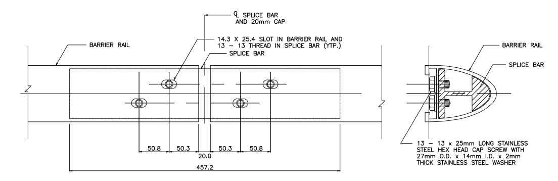
SPLICE BAR TO RAIL ASSEMBLY DETAIL
