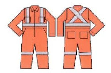
E8.3 In reference to E2.3 (Item No. 2), the reflective positioning requirements are as shown below:
