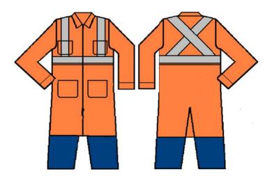
E8.5 In reference to E2.5 (Item No. 4), the reflective positioning requirements are shown below: (please note the required arm bands are missing in this image. Image is available of page 32 of the CSA catalogue).
