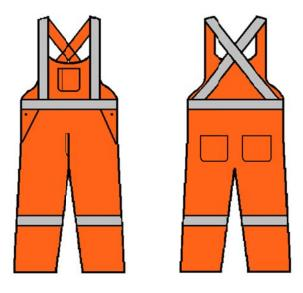
E8.4 In reference to E2.4 (Item No. 3), the reflective positioning requirements are as shown below: (please note the required arm bands are missing in this image. Image is available of page 32 of the CSA catalogue).
